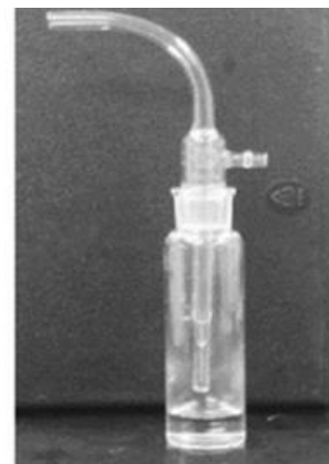
Figure 5: Air samples were taken with an AGI-30 impinger.
