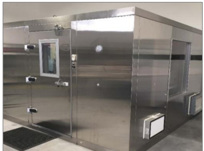
Figure 3: Stainless Steel Bioaerosol Test Chamber used for all Defend 1050 Device Testing. The Chamber has HEPA in/out, multiple bioaerosol sampling ports, decontamination, and pressure balance.
