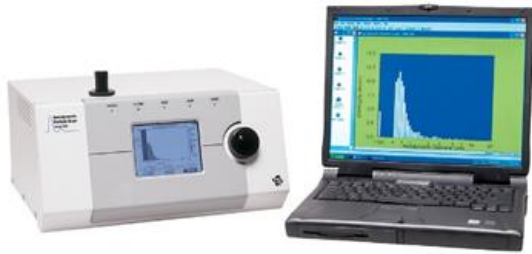
Figure 6. TSI Aerodynamic Particle Sizer (APS) model 3321 was used to measure the challenge-bioaerosol's total particle concentration and particle size distribution. The range is 0.54-20.0 \mu\text{m} aerodynamic diameter, with 1 particle/L detection limits.
